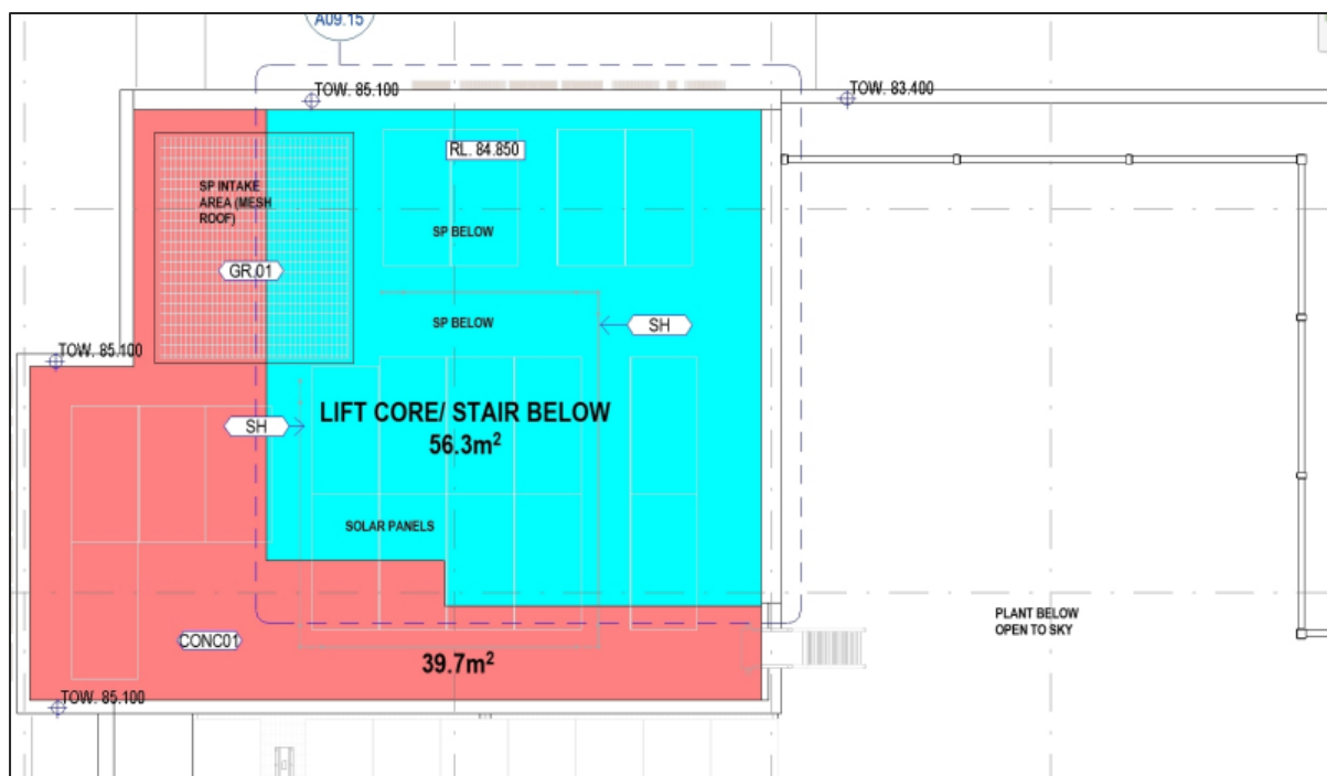
Figure 4 | The area of rooftop plant that meets the definition of a 'storey' and exceeds the height limit coloured red (Base source: RRtS Variation Request)
