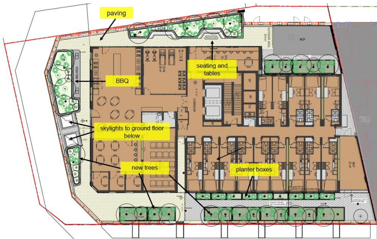
Figure 30 | Level 2 (podium rooftop) landscaping works (Base source: Applicant’s RRtS Landscape Plans)
