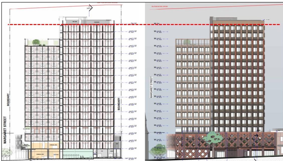
Figure 3 | Long section (left) and Regent Street elevation (right), indicating the 18-storey height plane (red dotted line) (Base source: RRtS Architectural Plans)
