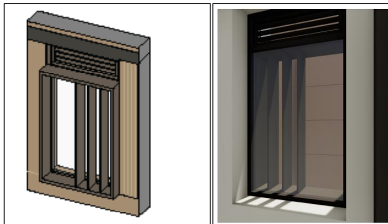
Figure 24 | External privacy fins proposed for north-eastern windows – left: 3D render, right: indicative view looking out (Source: RtS Urban Design Report)
